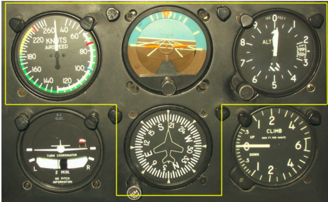
Figure 4: Detail of the on-board instrumentation of a P2002 JF, Tecnam. Note the arrangement of the essential tools described above. In the centre the artificial horizon, on the left the anemometer, on the right the altimeter, at the bottom the directional gyro.
