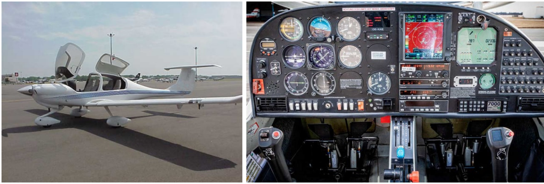
Figure 7: On the left, Diamond DA 40 180 (Diamond Aircraft Industries GMBH), on the right the cockpit. It is a single-engine model, equipped with a Textron Lycoming injection, variable pitch propeller and fixed landing gear.
